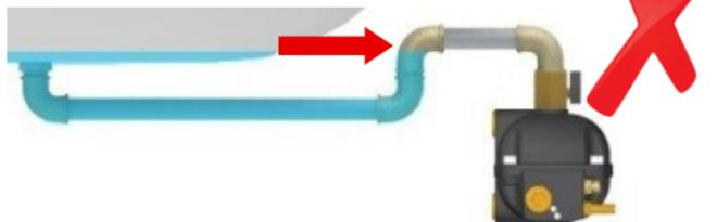
*The feed pipe must be horizontal or ideally at a downwards slope ( $>1^\circ$ ).*
