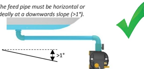
*If the downwards slope of the feed pipe is not sufficient, or if any other flow problem occurs, a venting line must be installed to prevent an air lock.*
