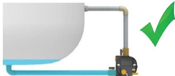
*Do not narrow the feed pipe when installing additional adapters or piping, these may cause air locks.*
